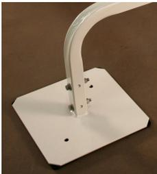
Our VRF Super Stand has four 12" x 12" feet, made from 7-gauge steel and 11-gauge steel tubing. It adjusts in 1/4" and 1/2" increments. This is done by rotating the foot 180 degrees. There are two 1/2" holes in each foot to secure the stand.
